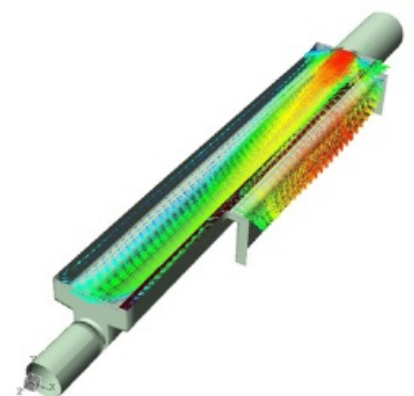
Figure 3: Flow in a revised geometry. A screened CSO based on the WaPUG guidelines [2]
