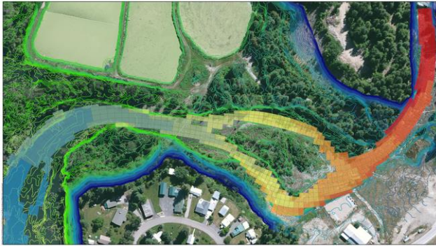
Area LiDAR and 2 Dimensional Model Grid Developed to Support Restoration Design Components and Alternatives
