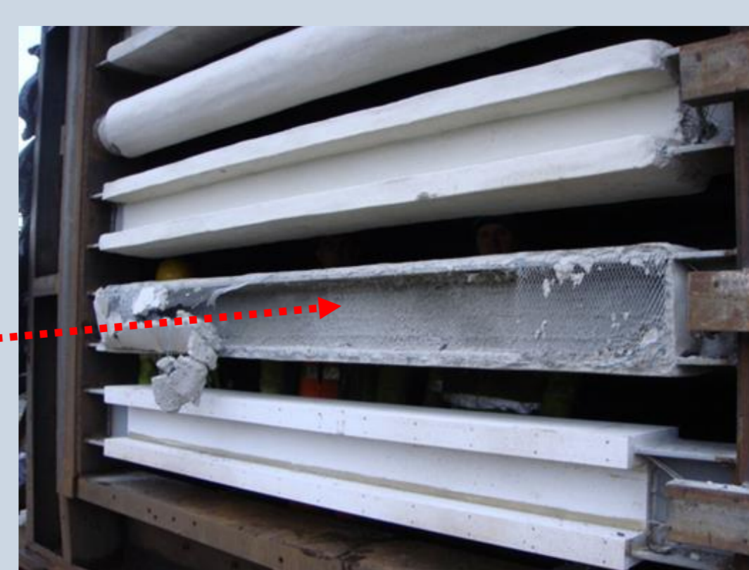
Figure 7a & 7b shows a blast loading response demonstration and the comparative performance of profile and boxed designs
