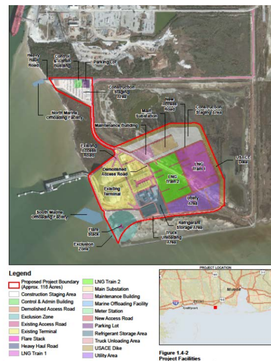
The planned plant site showing the two liquefaction trains and associated plant expansion areas
