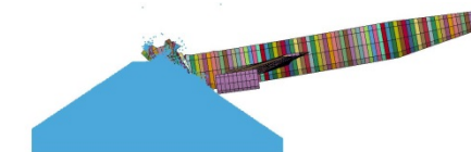
Figure 4: A plane hitting an earth berm used as protection of a nuclear facility – LS-DYNA smooth particle hydrodynamics representation for the soil material of the berm
