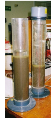
Figure 1: Bench tests determine empirical settling function
