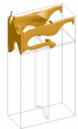
Figure 2: Delivery of Argon above a waste silo in a simulated fire event
