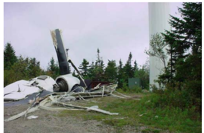
Turbine failure at Searsburg wind facility, Searsburg VT. Due to high wind conditions, a turbine blade hit the tower base causing the tower to buckle and the rotor assembly to crash to the ground (picture reproduced with permission from www.windaction.org )
