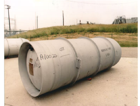
Figure 1: Typical UF 6 storage cylinder
