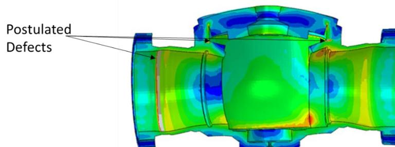
FE predicted deformed shape and von Mises stress contours of the valve with postulated cracks
