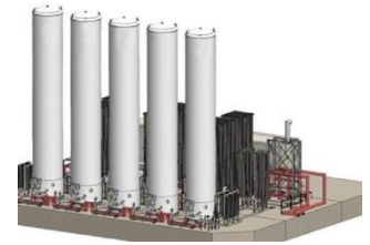
Figure 1: Nitrogen Deluge System
